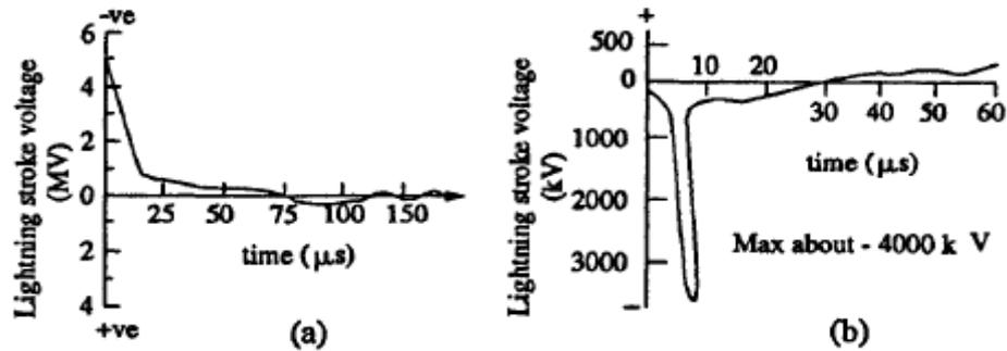
**FIG 5 Typical lightning stroke voltage on a transmission line without ground wire**
