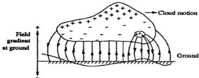
**Fig.1 Probable field gradient near the ground corresponding to the probable charge distribution in a cloud.**
