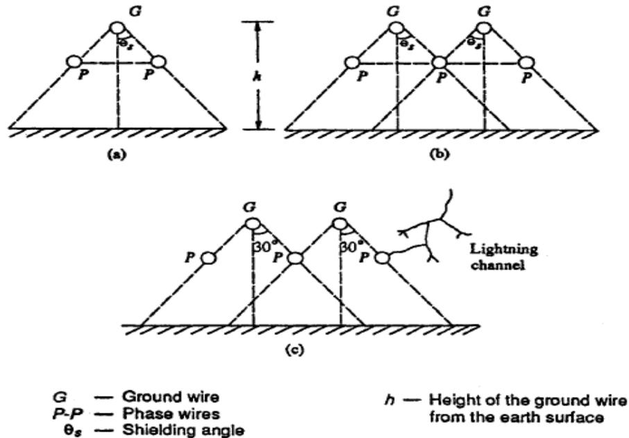
**FIG 8 Shielding arrangement of overhead lines by ground wires**
