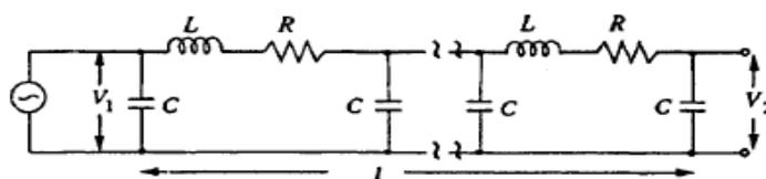
$L, R$  and  $C$  — Inductance, resistance and capacitance per unit length of the line
