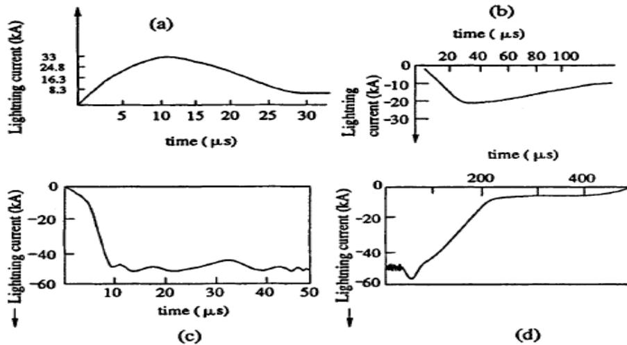
**FIG 4:- Typical lightning current oscillograms**
