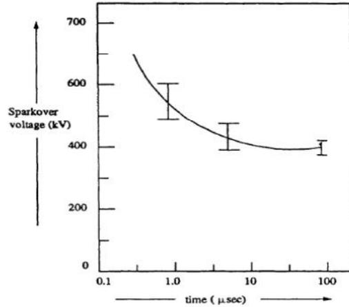
**FIG Volt-time characteristic of a standard rod-rod gap**
