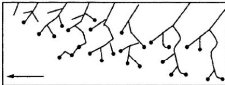
**FIG 3 Propagation of a stepped leader stroke from a cloud (• Bright tips recorded)**
